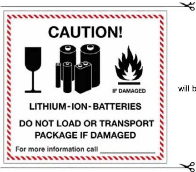
The link to Safe transportation of batteries link will bring up this label which will be required to be printed out and stuck onto the outside of the packaging
